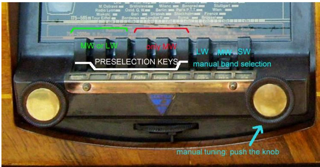
NOTE 1: for manual tuning, push one of the last three keys (first: LW; second: MW; third: SW), then push the tuning knob until it locks; finally, to change stations, turn the tuning knob. The subsequent activation of one of the first six preselection keys causes the release of the manual tuning knob.
